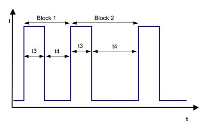
Block1: special locked rotor protection: 5 cycles t3 / t4 = 0.6 s / 0.5 s Block2: locked rotor protection t3 / t4 = 0.6 s / 10 s
