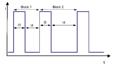
Block1: special locked rotor protection: 5 cycles t3 / t4 = 0,6 s / 0,5 s Block2: locked rotor protection t3 / t4 = 0,6 s / 10 s
