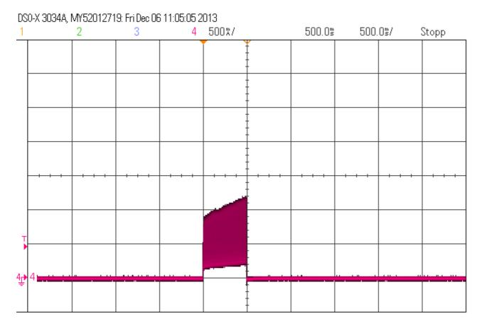
Locked rotor current @ 60 V (I = 500mA/div ; t = 500ms/div)
